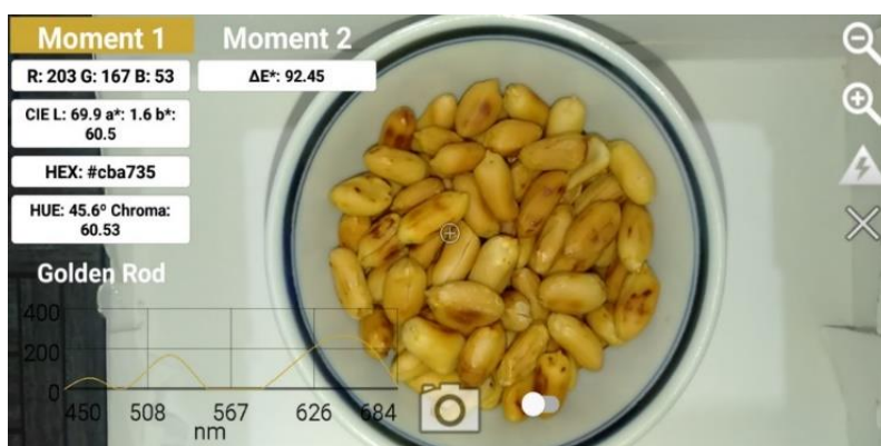
Figure 7. The CIE L* capture of 100-gram peanut from one of the samples roasted in 18 minutes.
